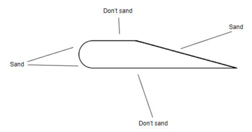
This is an oversimplification of how airfoils are shaped, but it helps to demonstrate where the wing should actually be sanded.
